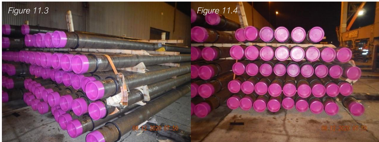
Ratchet Straps and wedges installed – Side profile of stow
