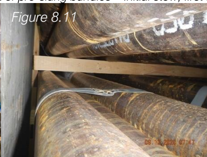
5 rows of separating dunnage - Stow of pipes – Top layer part row of 6 bundles
