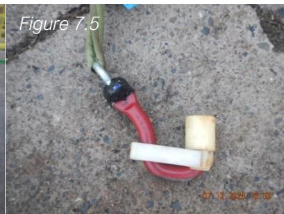
Spreader Frame - Pipe hook with polyurethane cover – Lifting method
