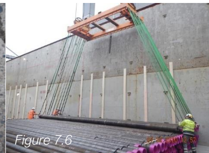
Spreader Frame - Pipe hook with polyurethane cover – Lifting method
