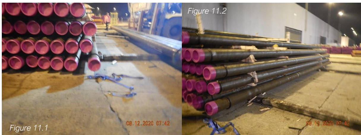
Picture taken on arrival at the site, 1 min after event – Broken dunnage frame
