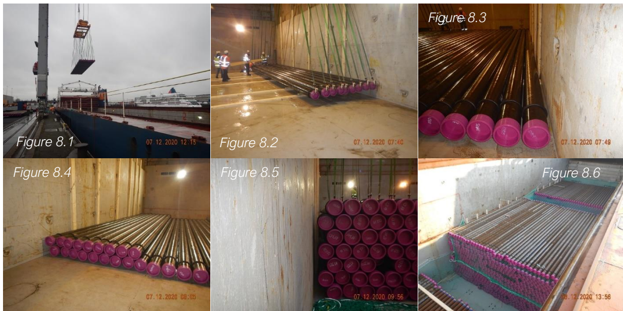
Stow of 10' Pipe, Stacks 2, 3 & 4
