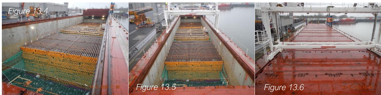
Final Cargo arrangement and securing of hatch covers
