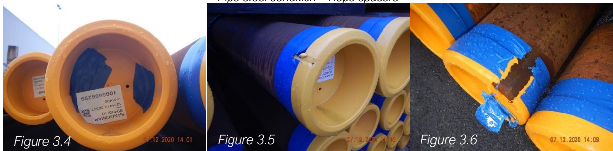
End caps with repairs – Damage to end caps and tape
