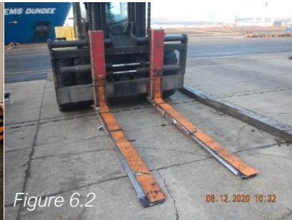
Kocks Gantry Crane – Hyster 20-12 Heavy Duty Fork Lift – Protection fitted to fork lift teeth
