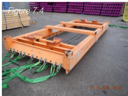
Spreader Frame - Pipe hook with polyurethane cover – Lifting method
