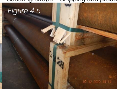
Moisture below end cap – Minor damage to crating
