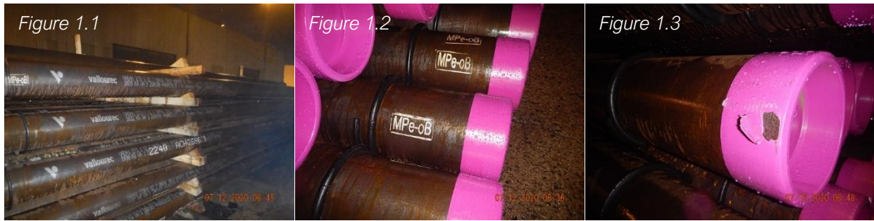
Figure 1.1 Figure 1.2 Figure 1.3 Pipe Markings – Spacers, End Caps & Test Marking – Damage to end cap
