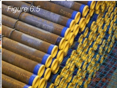
Pipe pre-loading stow and checks – tape repairs to [redacted] and [redacted] Pipes
