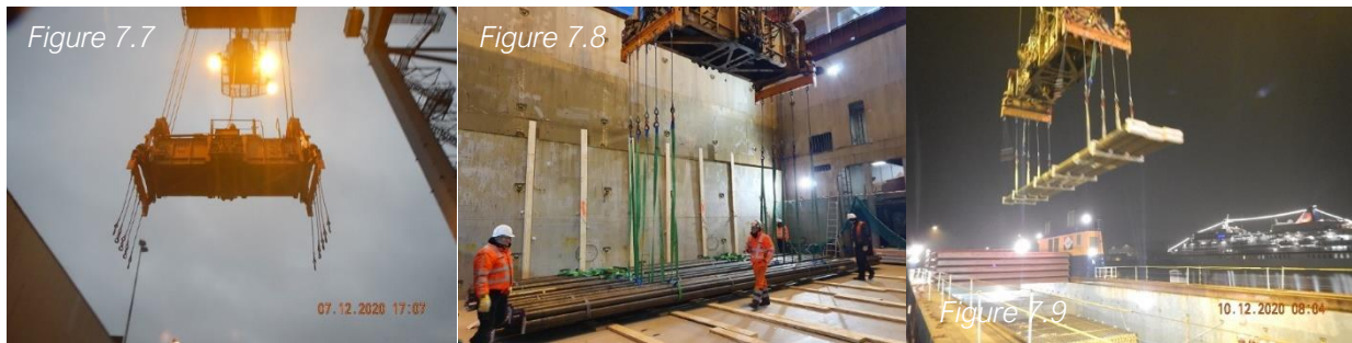
Container lifter fitted with securing bars – Slung bundles – Slung crated pipes
