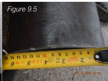
No deformation – mark to 10463/81518165 – measured at 20mm
