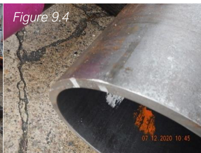
No deformation – mark to 10463/81518165 – measured at 20mm
