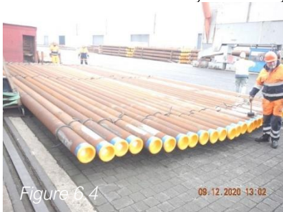
Pipe pre-loading stow and checks – tape repairs to [redacted] and [redacted] Pipes
