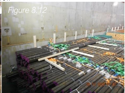
5 rows of separating dunnage - Stow of pipes – Top layer part row of 6 bundles
