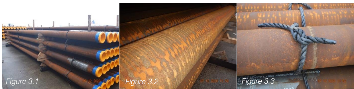
Pipe steel condition – Rope spacers
