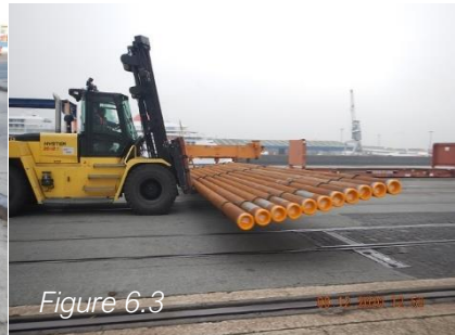
Kocks Gantry Crane – Hyster 20-12 Heavy Duty Fork Lift – Protection fitted to fork lift teeth
