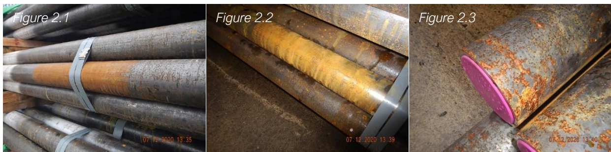
Figure 2.1 Figure 2.2 Figure 2.3 Bundle straps – Steel condition, light oxidation
